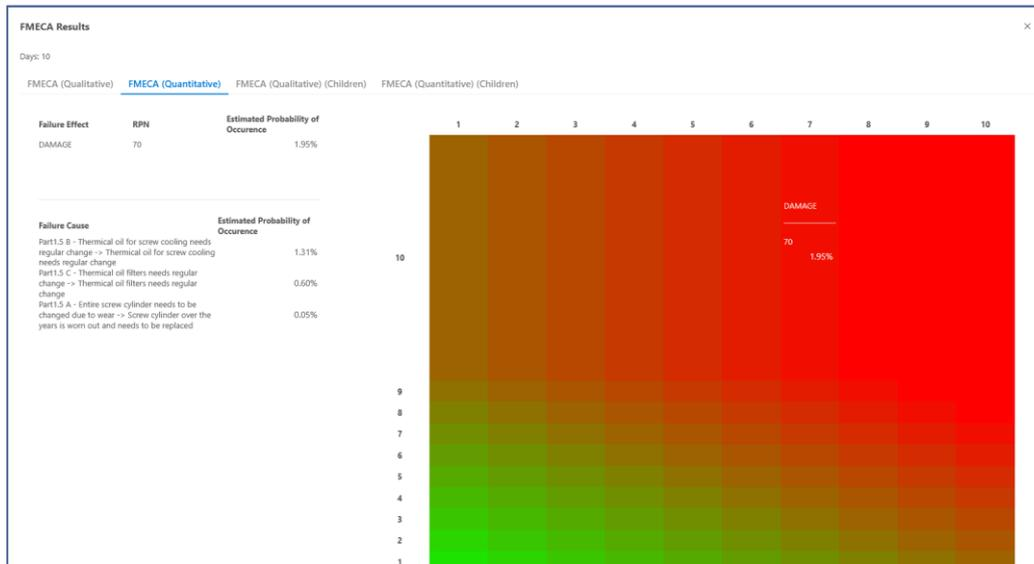
Figure 2: FMECA results in Heat Matrixes
