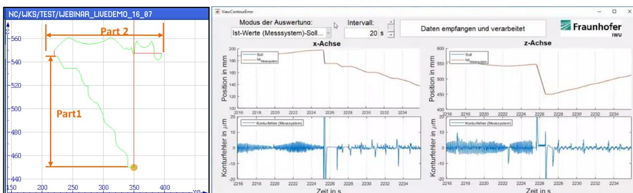
Figure 1: Demo program for the demonstration of the digital twin for path accuracy (left) and graphical user interface depicting the current path accuracy (right)
