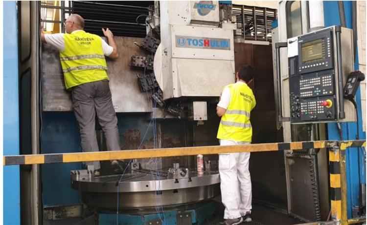
Figure 2: Preliminary experiments for identifying the machine tool dynamics of the industrial lathe at TOSHULIN
